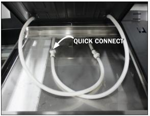
Fig. 19 Quick connect engaged
