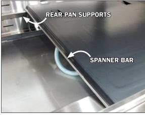
Fig. 16 Spanner bar & rear pan support
