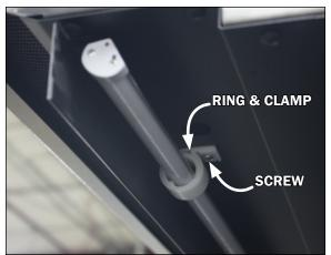
Fig. 12 LED light & ring/clamp
